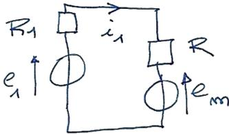
$$e_1 = (R_1 + R) i_1 + \phi_0 \omega \quad (1), \text{ car } e_m = \phi_0 \omega.$$
