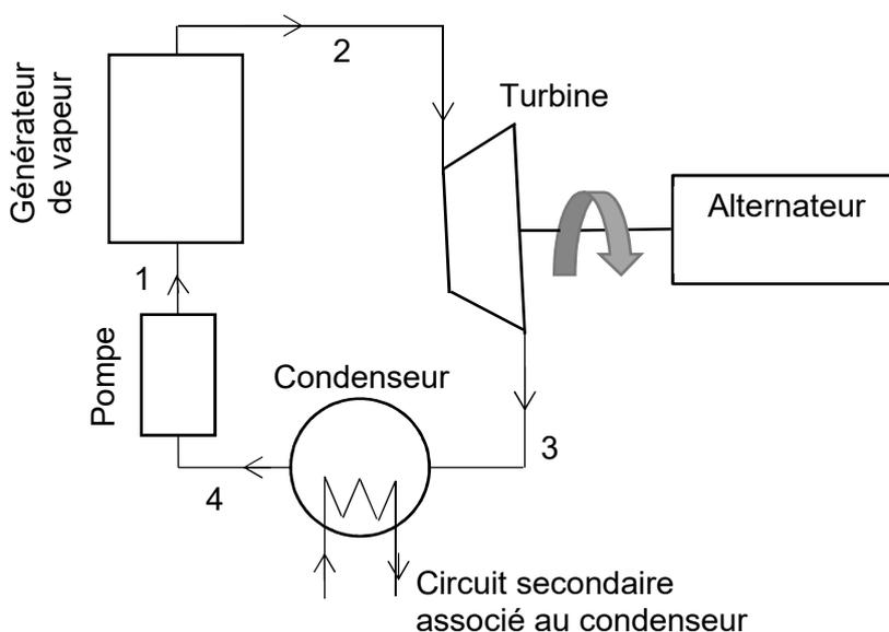
**Figure 6** - Installation motrice
